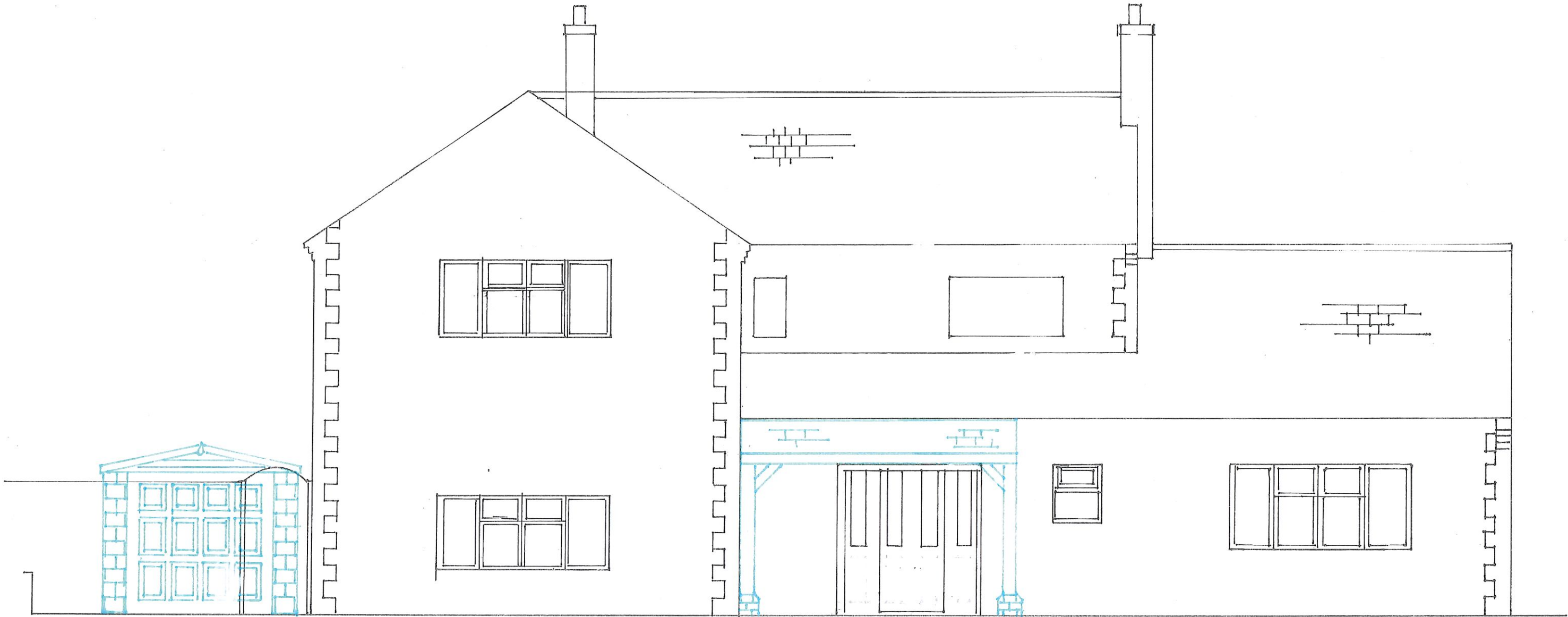
OAK FRAME PORCH ON BRICK PILLARS WITH SHINGLE ROOF
