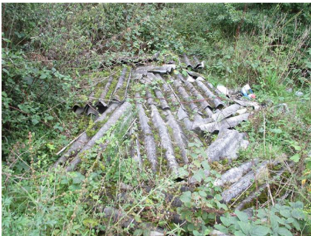
Plate 24: Possible ACM found in the north east area of the site near Oak Road.
