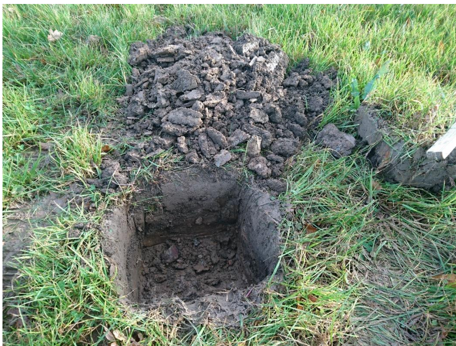
Figure 2-10: Trial Pit in Field 1C – terminated due to low observed rates of infiltration
