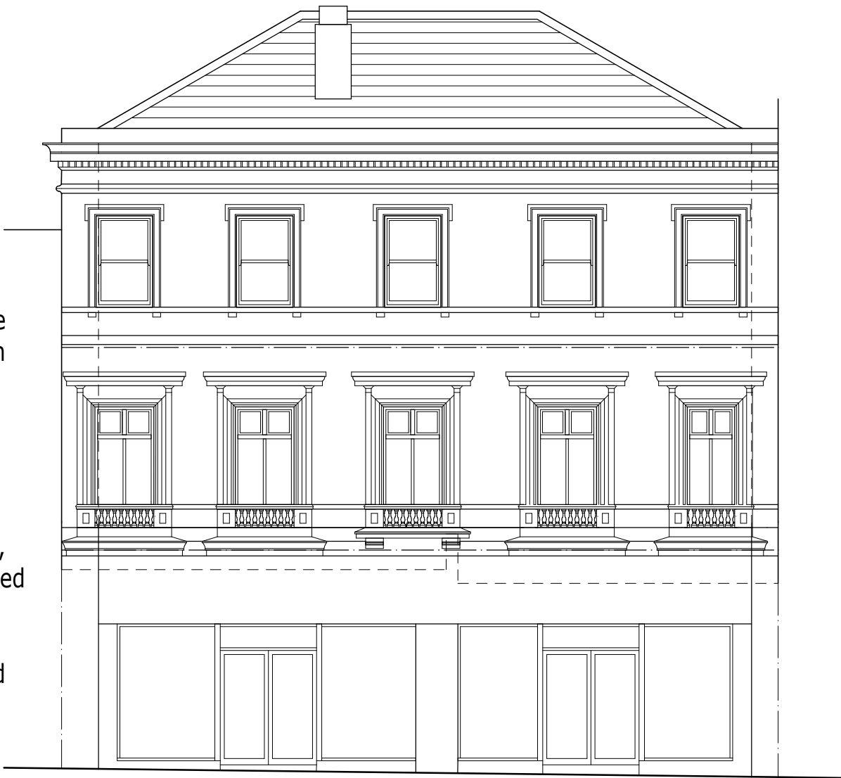
PROPOSED FRONT ELEVATION - PARAPET REMOVED TO REVEAL FIRST FLOOR OPENINGS.
