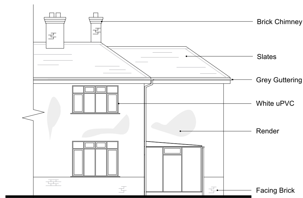
Existing Side Elevation View A - 1:100
