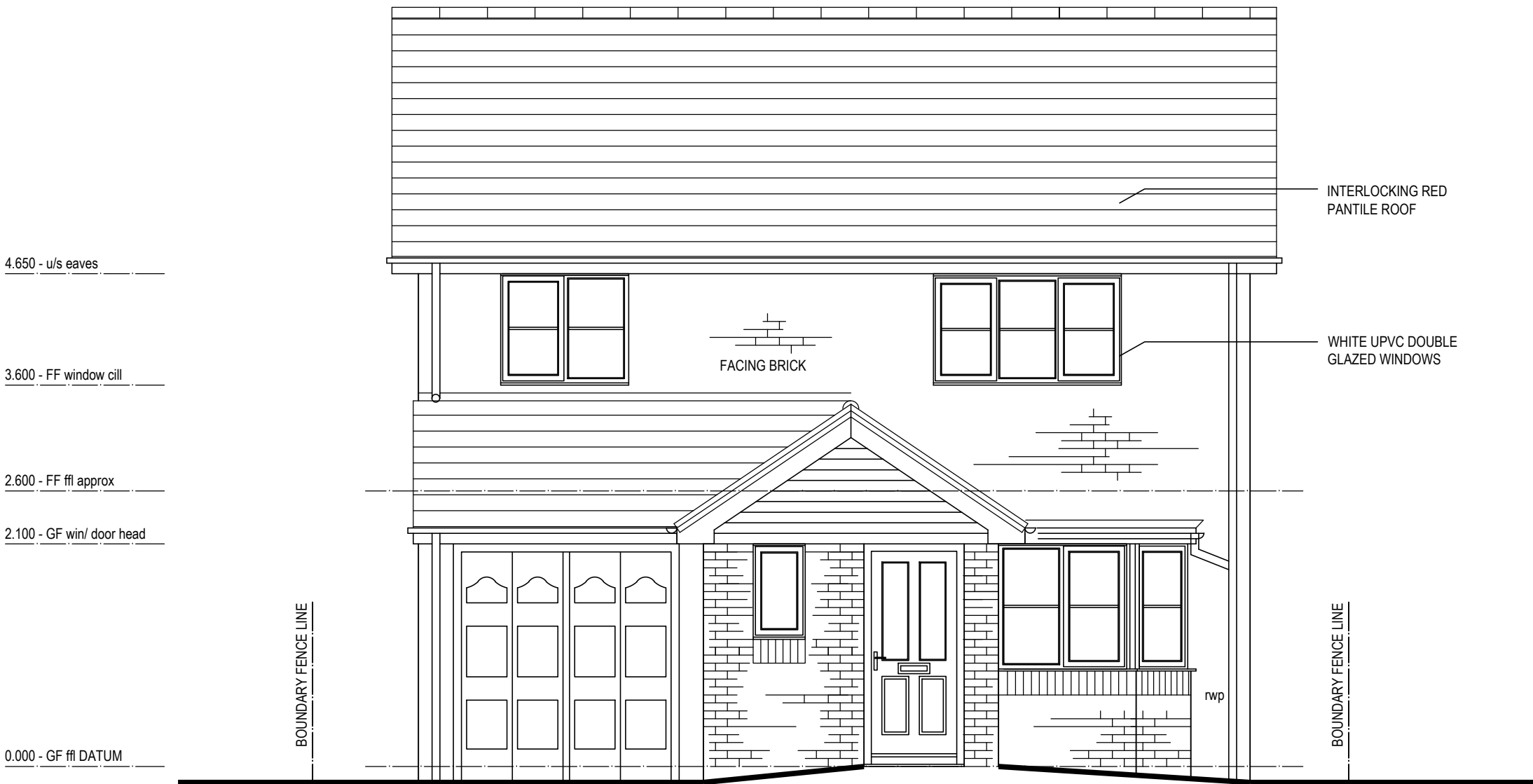
FRONT ELEVATION - FACING SOUTH-EAST
