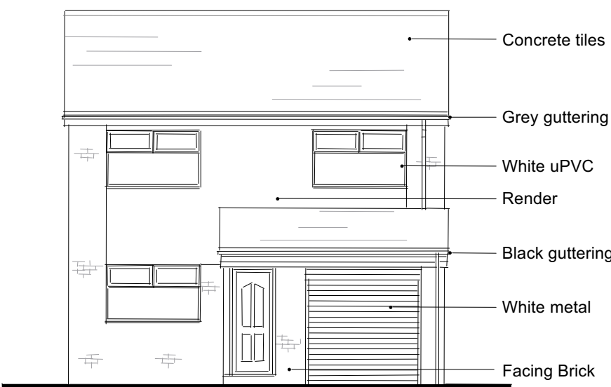
Existing Front Elevation View A - 1:100
