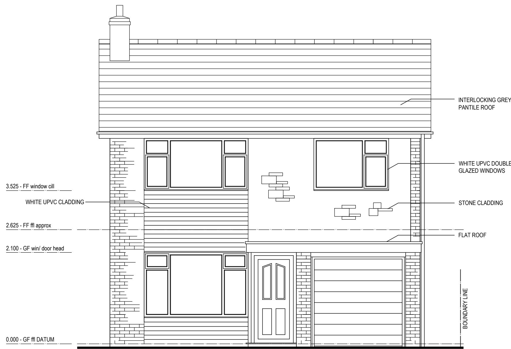
FRONT ELEVATION - FACING SOUTH
