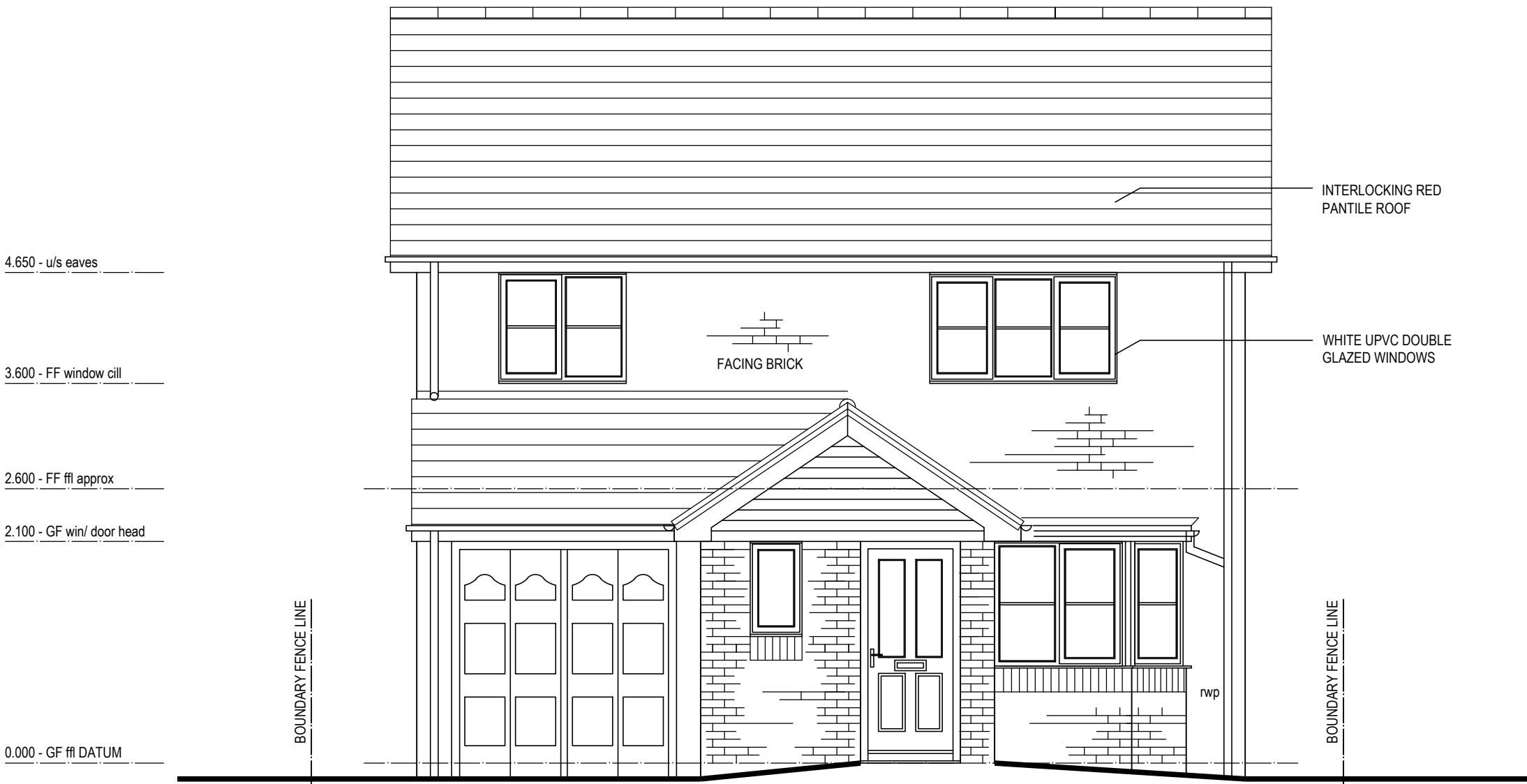
FRONT ELEVATION - FACING SOUTH-EAST
