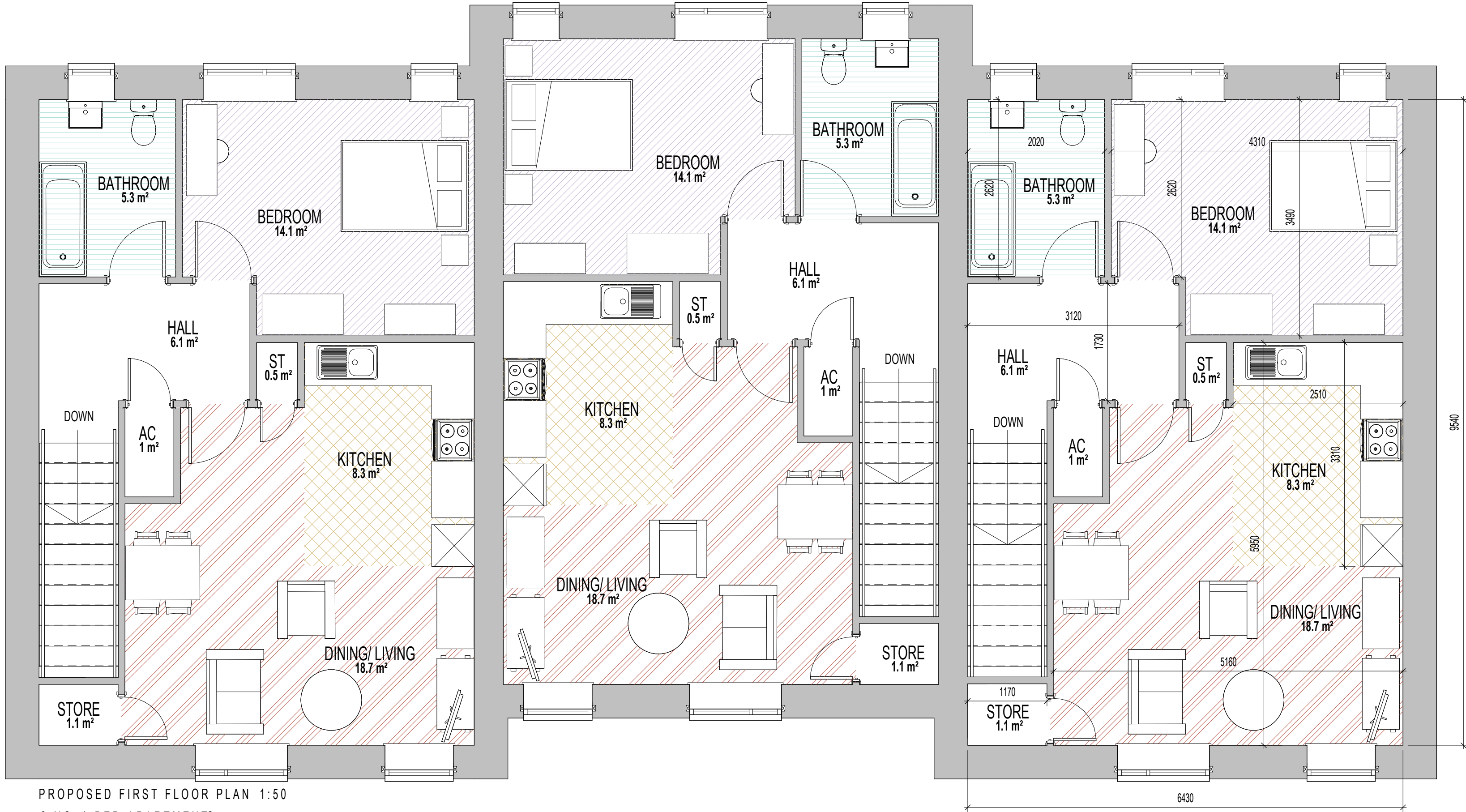
PROPOSED FIRST FLOOR PLAN 1:50 3 NO. 1 BED APARTMENTS
