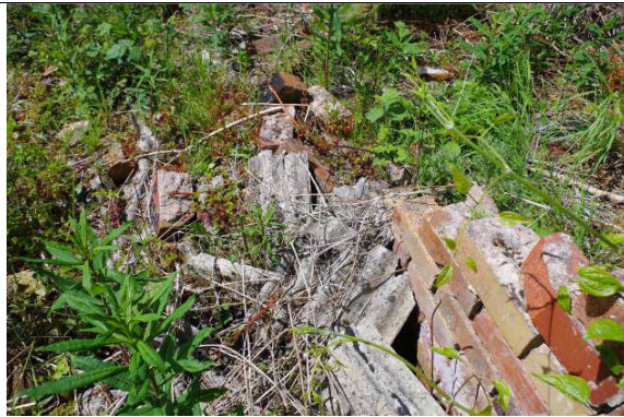
asbestos cement sheet fragments
