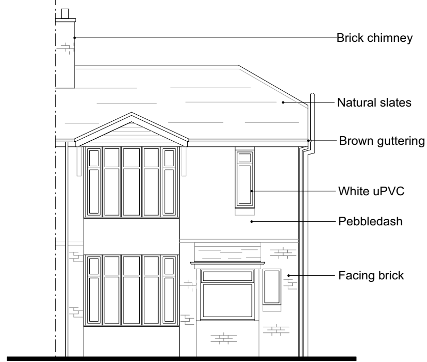
Existing Front Elevation View A - 1:100
