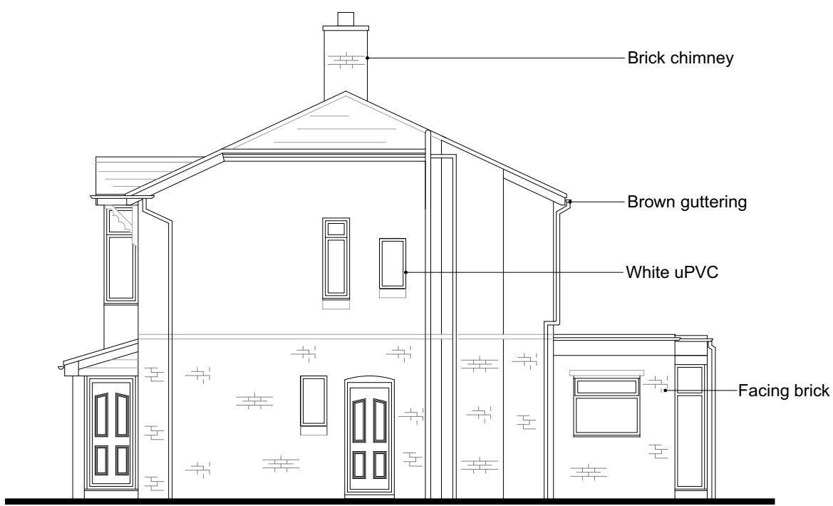
Existing Side Elevation View B - 1:100
