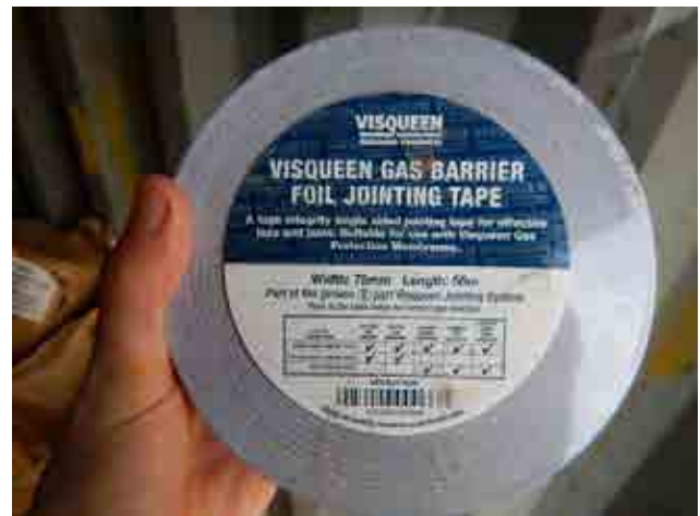
Photographs 10 and 11: Confirm ancillary products utilised in the gas membrane installation.
