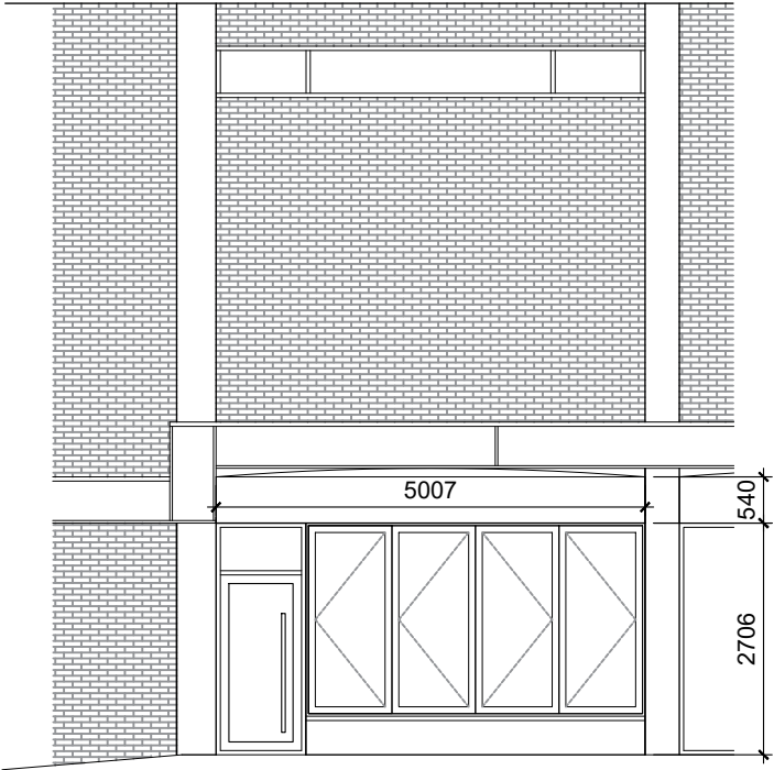
EXISTING FRONT ELEVATION
