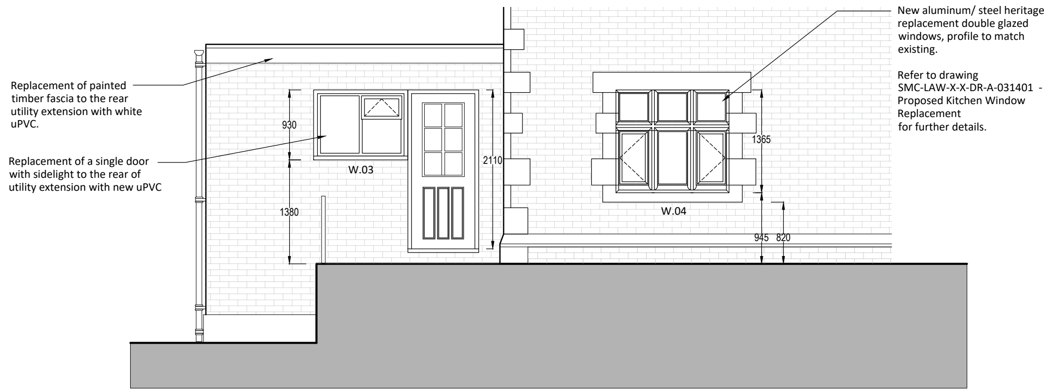
Rear Extension Elevation 02 1:50
