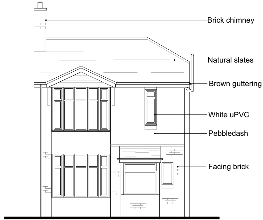
Existing Front Elevation View A - 1:100
