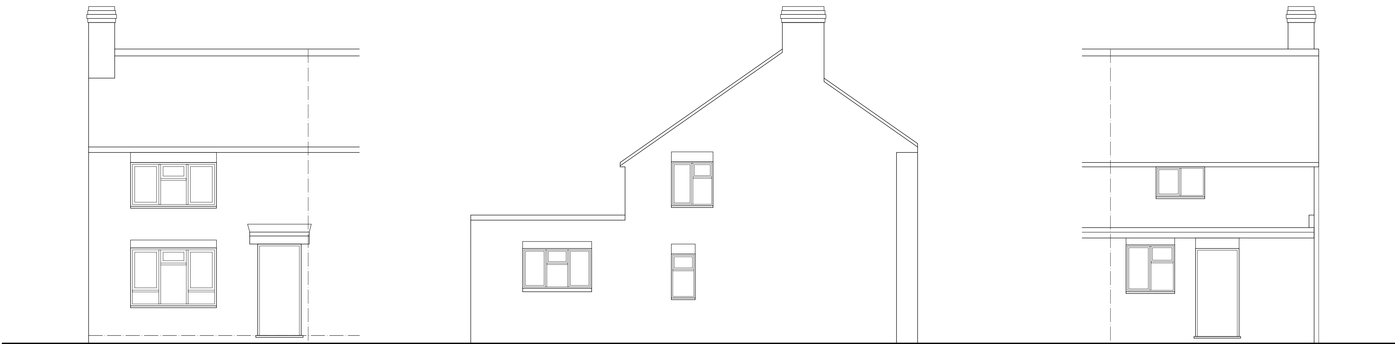
EXISTING FRONT ELEVATION.
