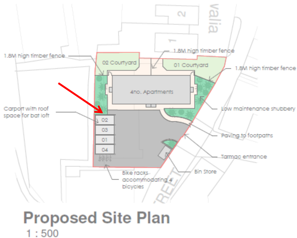
Figure 6.5. Showing position of integral bat box
