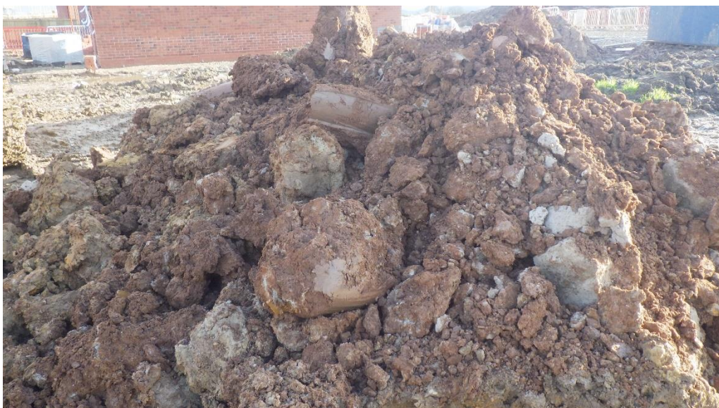
Photo 6 – Arising's from Trial Pit 203
