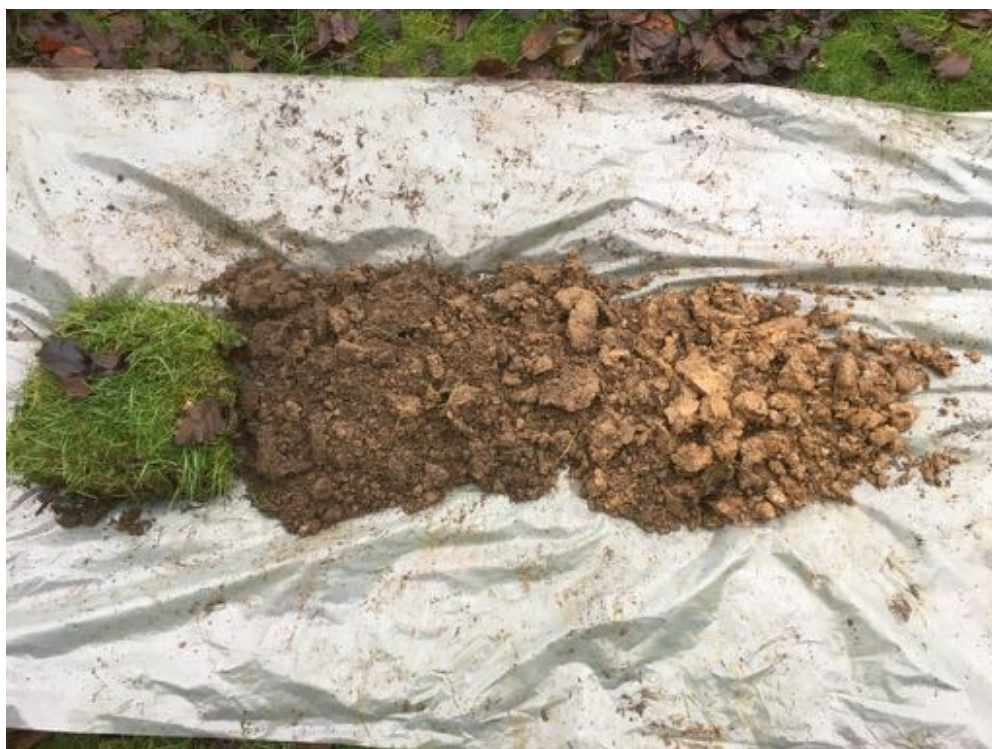
Photograph 37 Description: Soil sequence encountered at HP06 Date: 18/12/2019 Location: Central part of the orchard area
