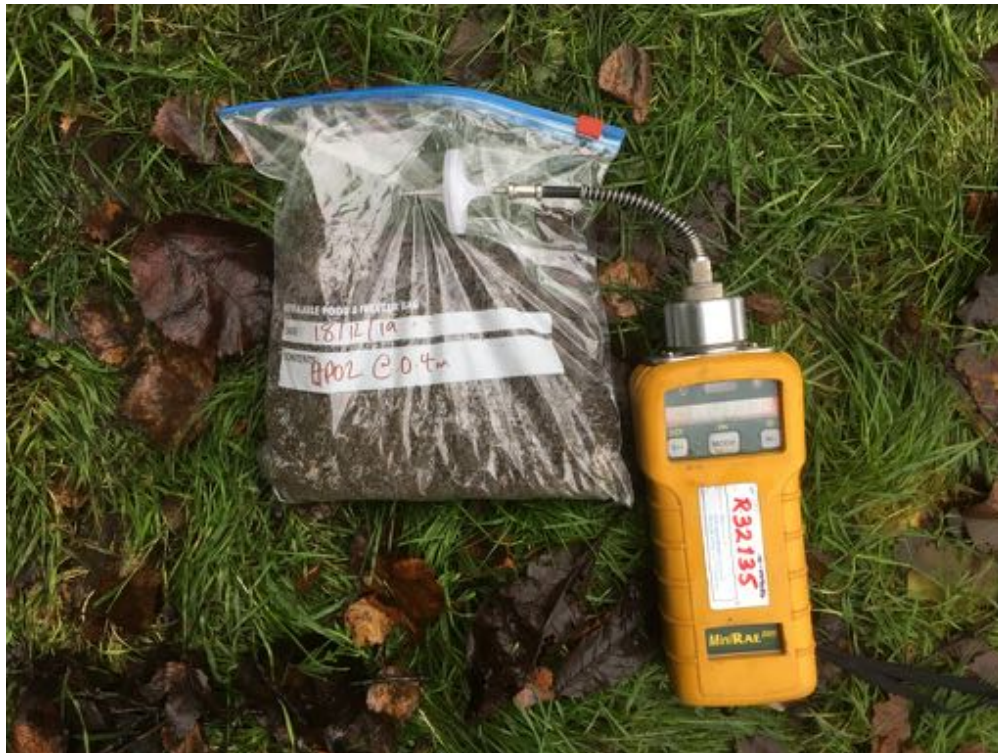
Photograph 55 Description: Example of soil sample PID headspace testing Date: 18/12/2019
