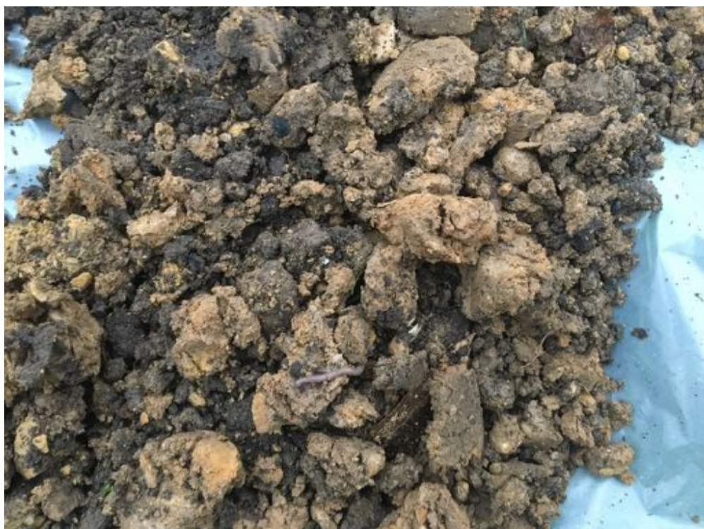
Photograph 17 Description: Reworked Till encountered at HP01 Date: 18/12/2019 Location: North-western corner of the Site
