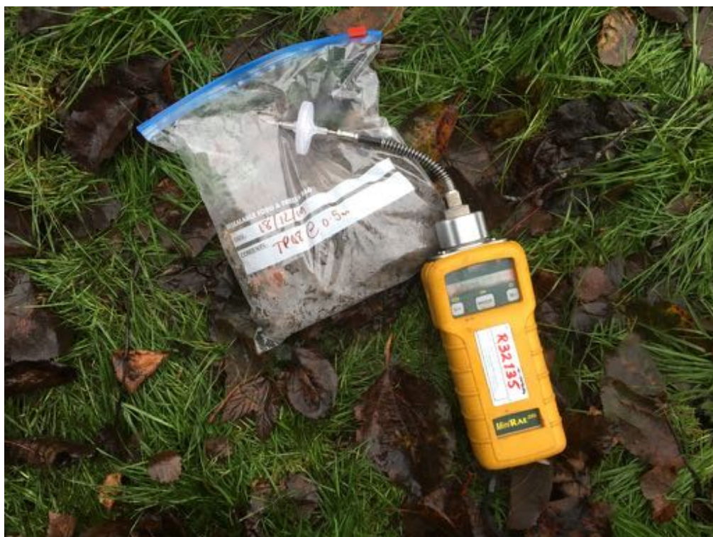
Photograph 57 Description: Example of soil sample PID headspace testing Date: 18/12/2019
