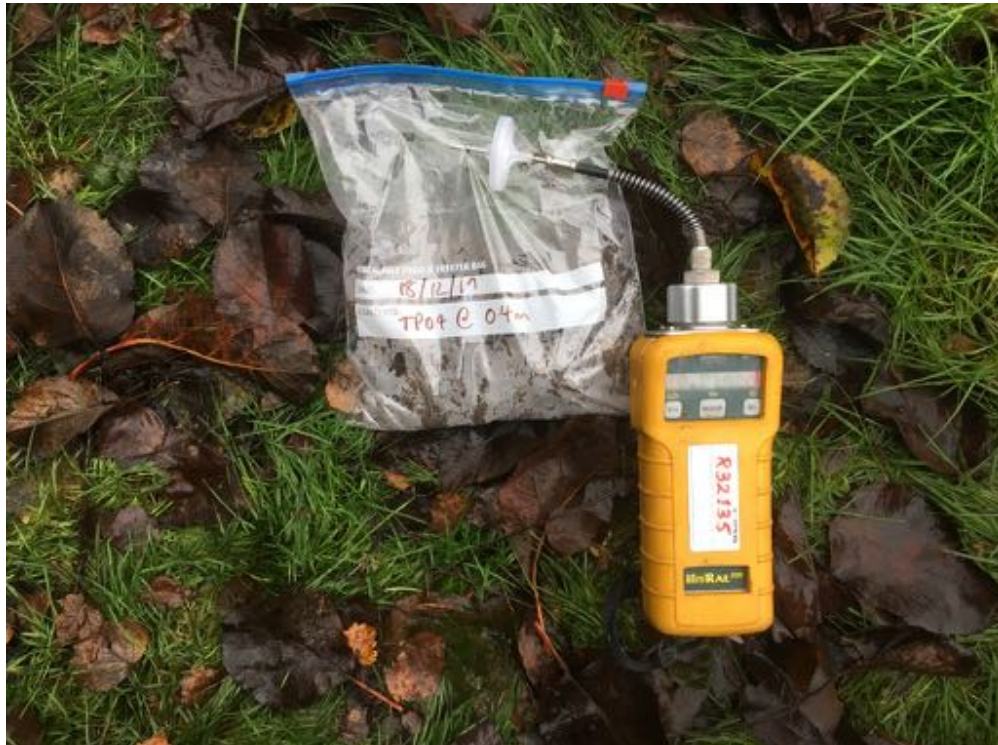
Photograph 56 Description: Example of soil sample PID headspace testing Date: 18/12/2019
