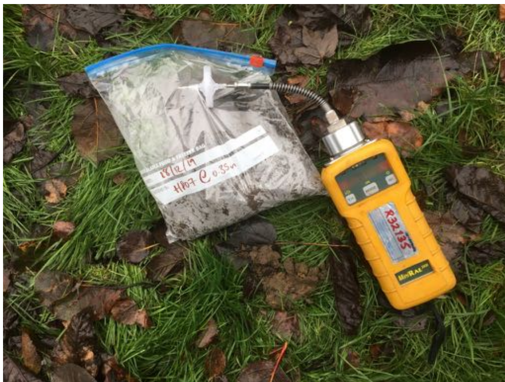
Photograph 58 Description: Example of soil sample PID headspace testing Date: 18/12/2019
