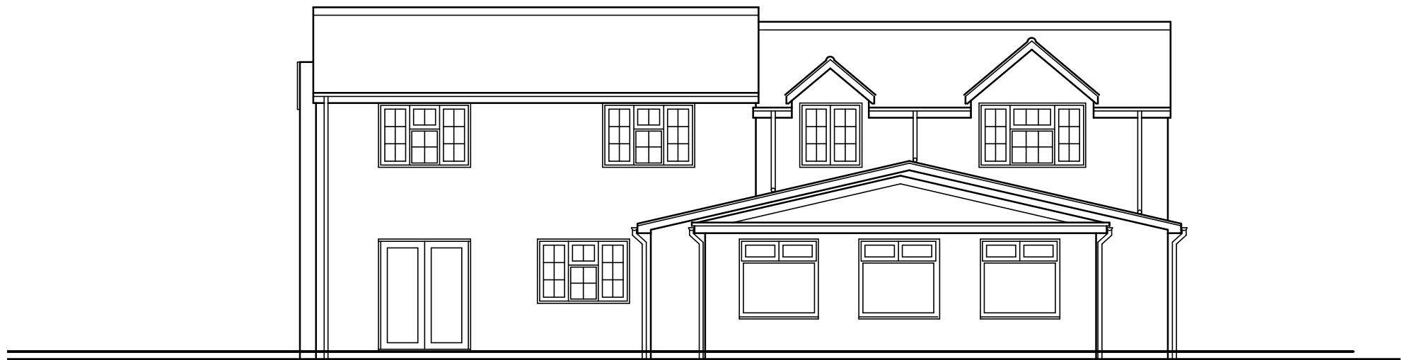
Rear Elevation as Existing
