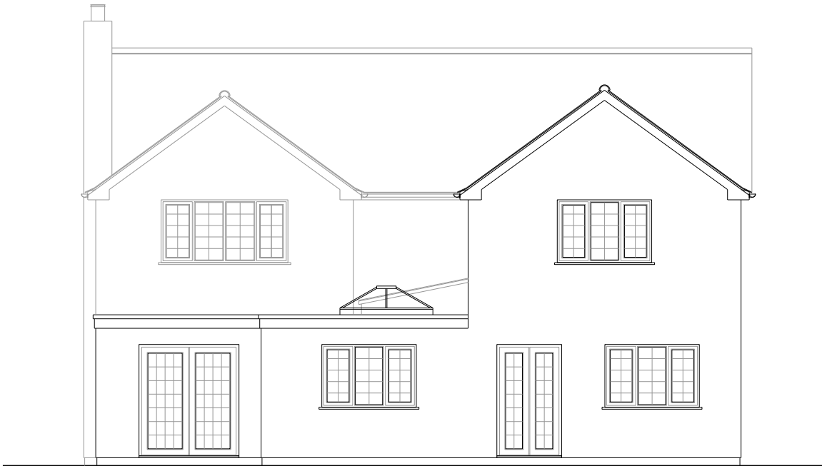
EXISTING REAR ELEVATION
