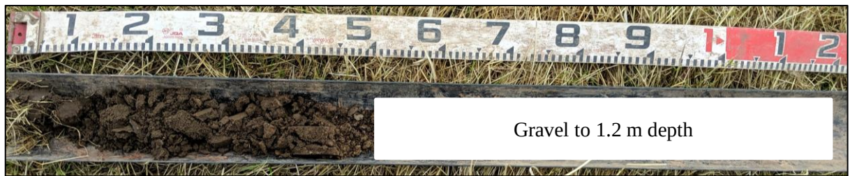
Photo 1. Boring location 14 – Profile of Soil Type 1
