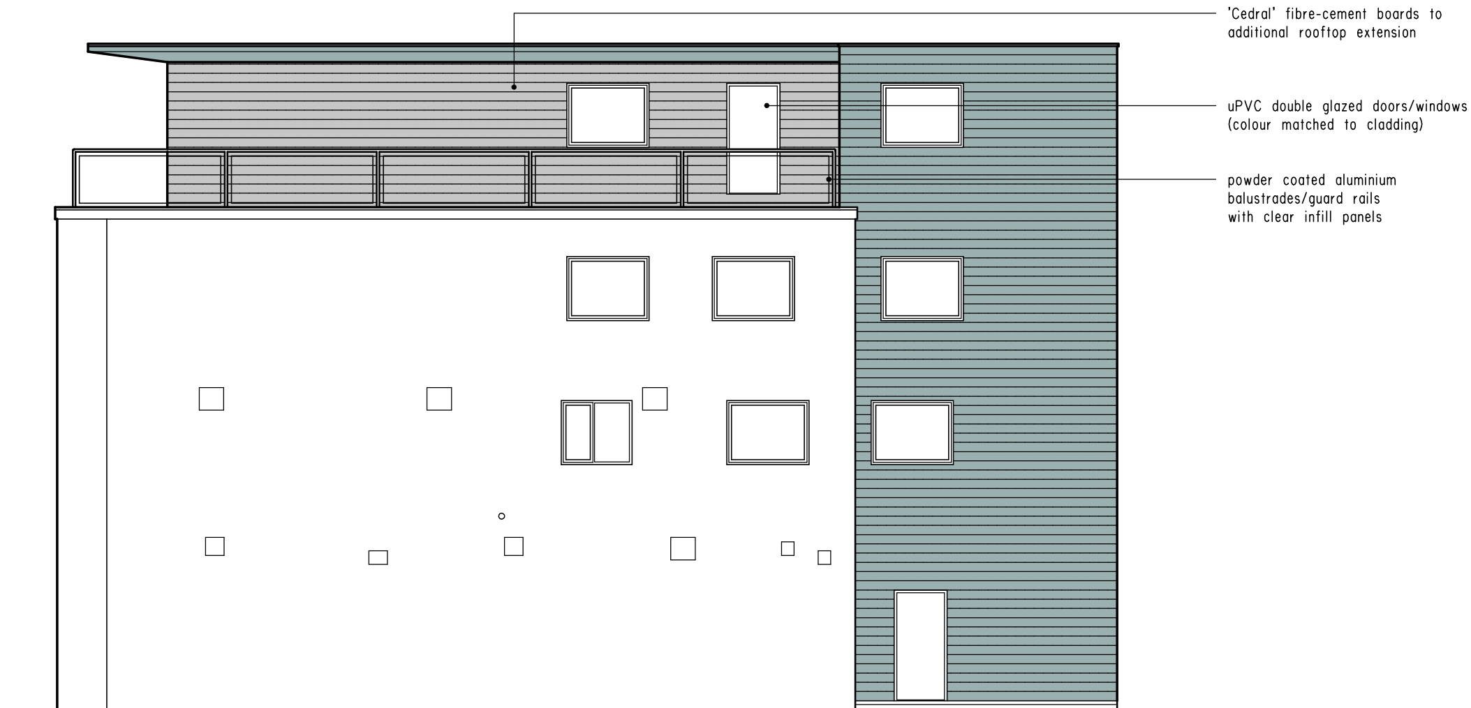
SIDE (NORTH-EAST) ELEVATION
