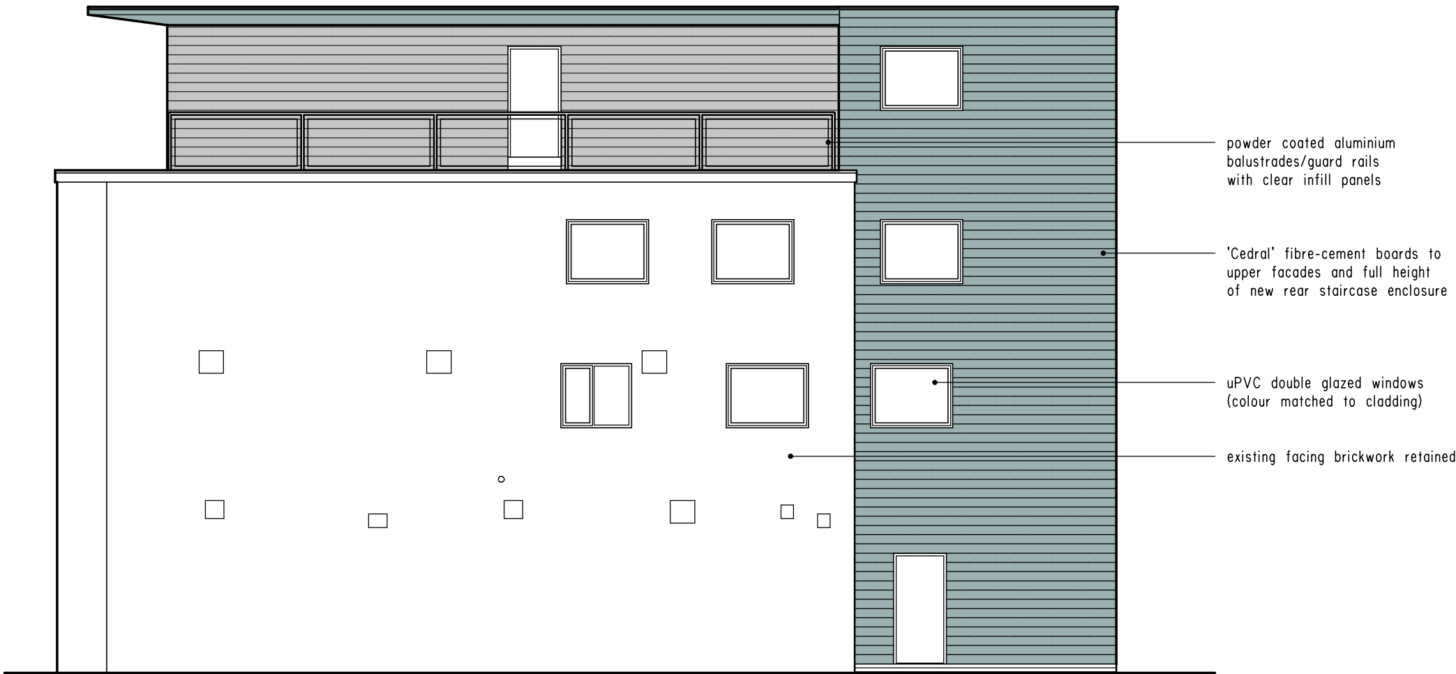
SIDE (NORTH-EAST) ELEVATION
