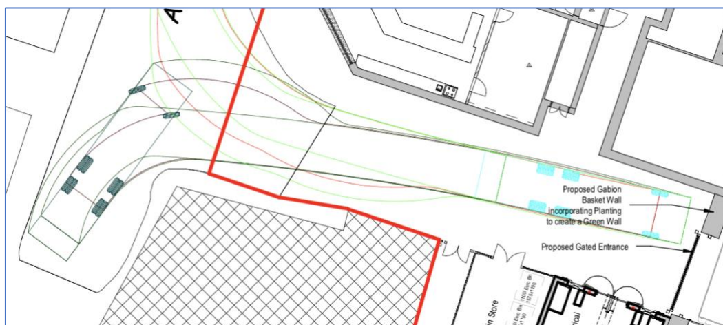
Plan 7 – Vehicle tracking for 11.2 refuse vehicle
