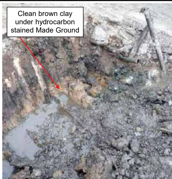
Photograph Three - Shallow hydrocarbon impacted soil and perched water. Underlying clean clay TP101
