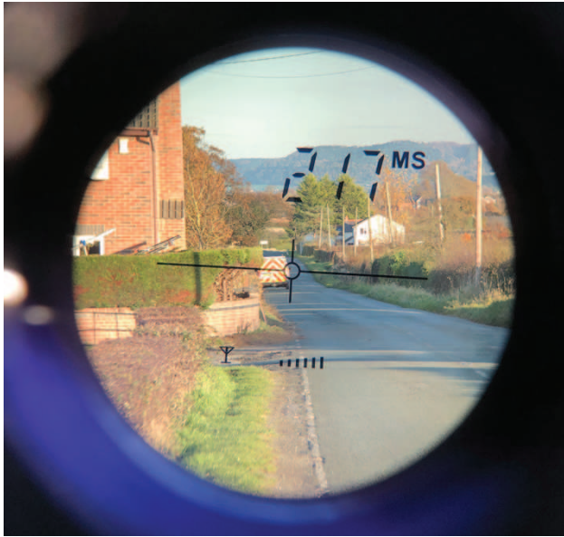
Fig 3: Taken from a location slightly closer to the road to enable the laser range finder to identify the van (217m distance).
