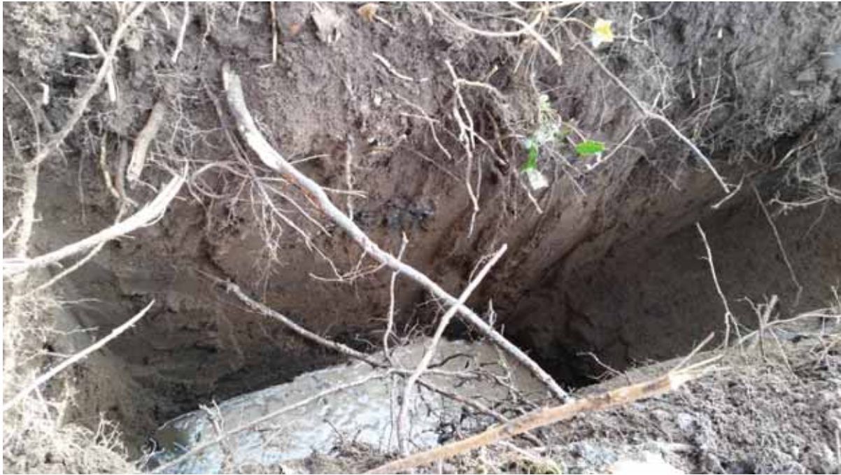
Photograph 21: Shows TP02 to depth of 1.8m and sides of trial pit.
