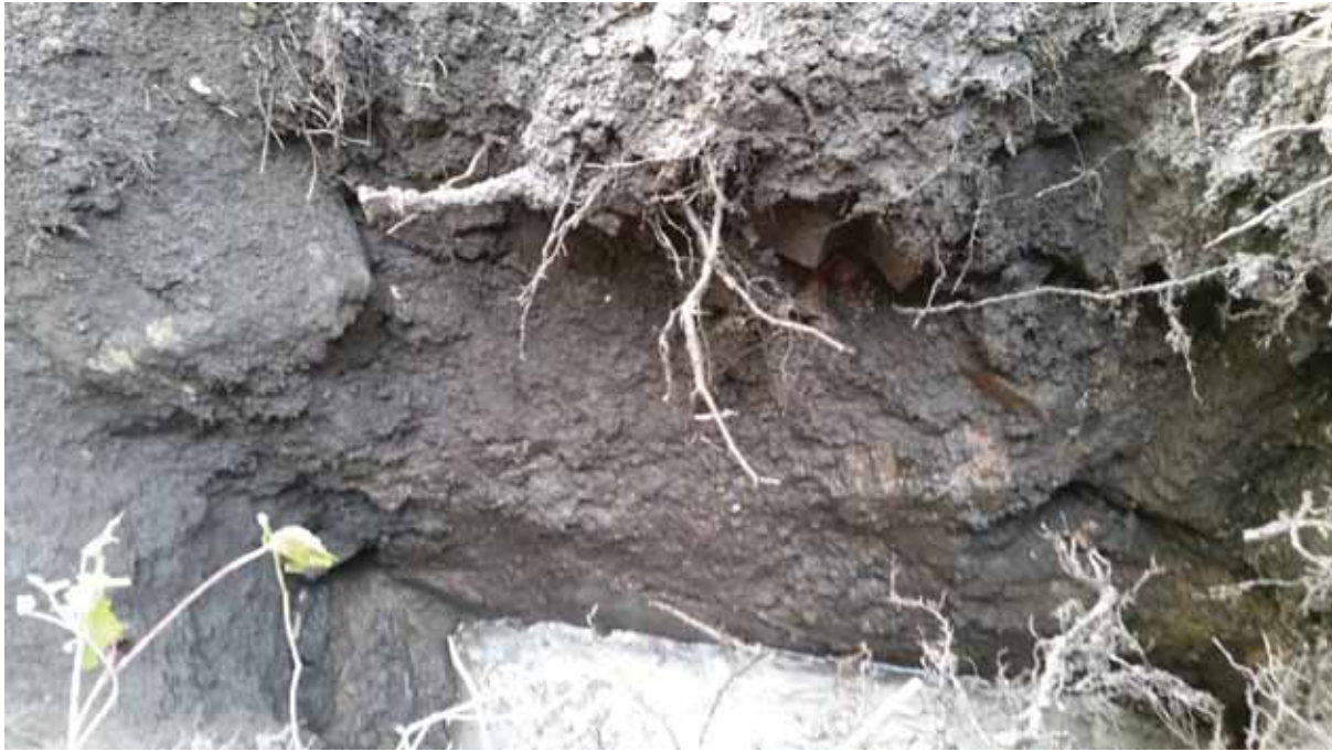
Photograph 24: Shows TP03 to a depth of 2m and sides of the trial pit.
