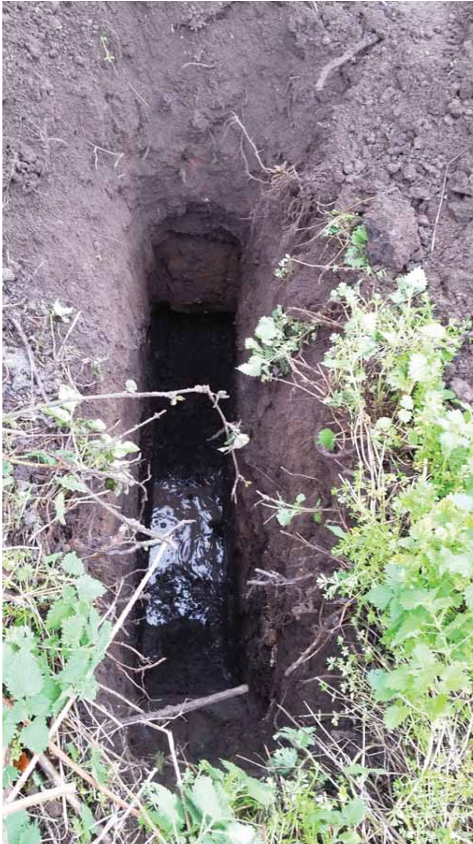
Photograph 15: Shows TP01 to depth of 2.1m
