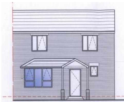
Figure 3. Proposed Front Elevation – Single Storey Porch Extension
