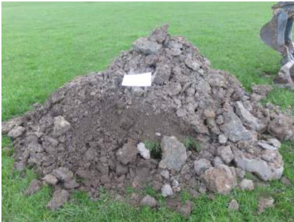
Photo 24 – Arising's from Trial Pit 12
