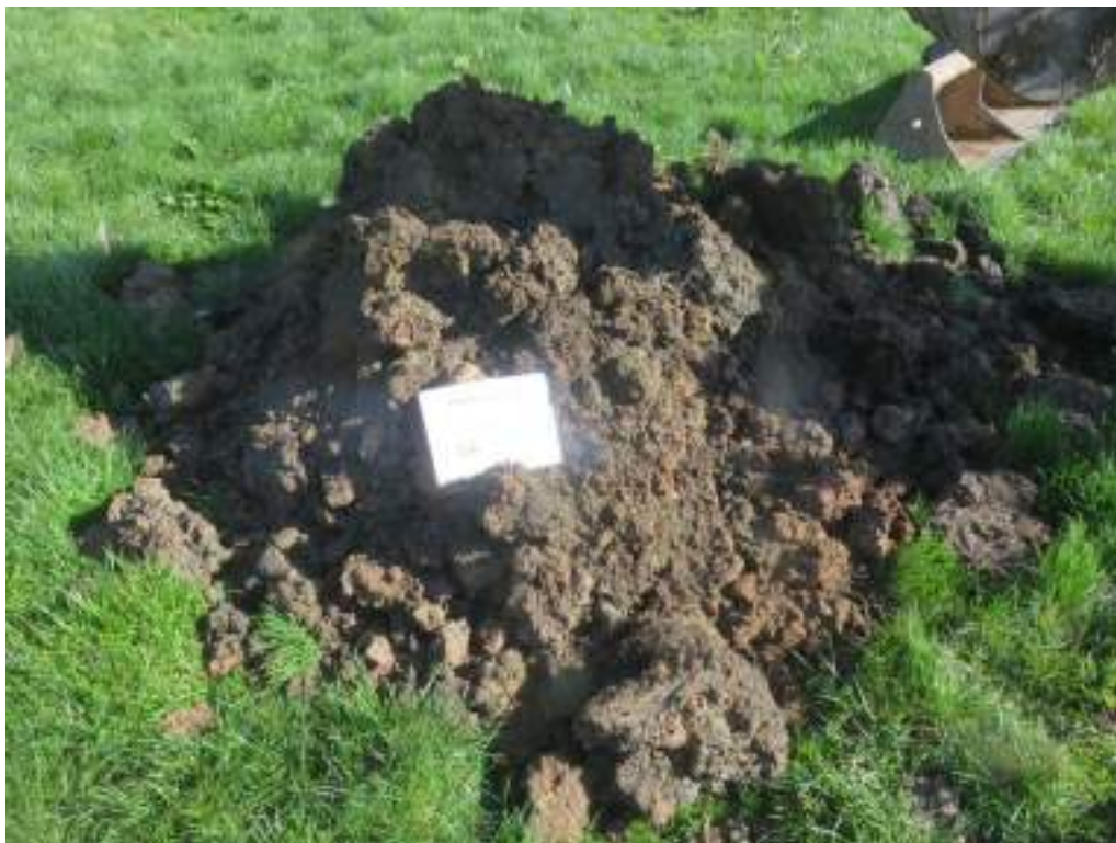
Photo 64 – Arising's from Trial Pit 32
