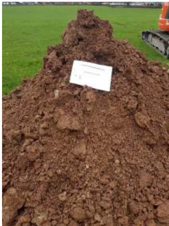
Photo 2 – Arising's from Trial Pit 01
