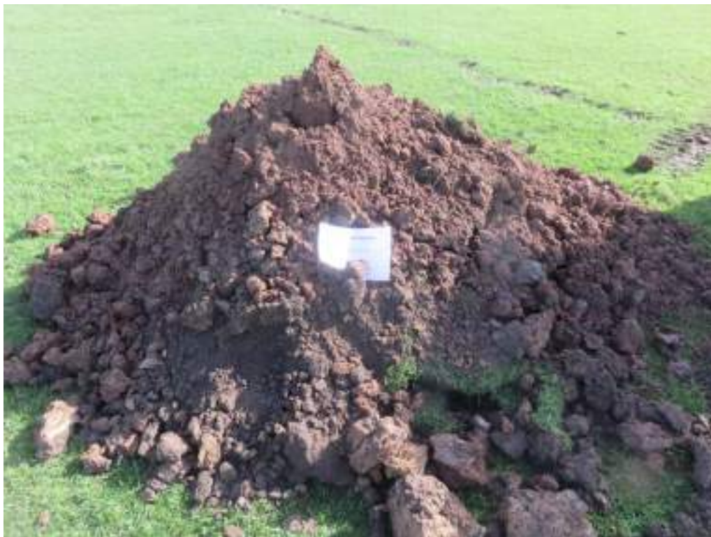
Photo 50 – Arising's from Trial Pit 25
