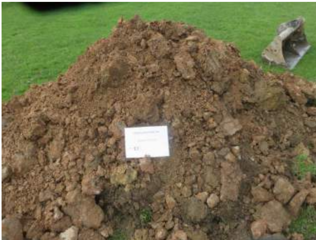
Photo 36 – Arising's from Trial Pit 18
