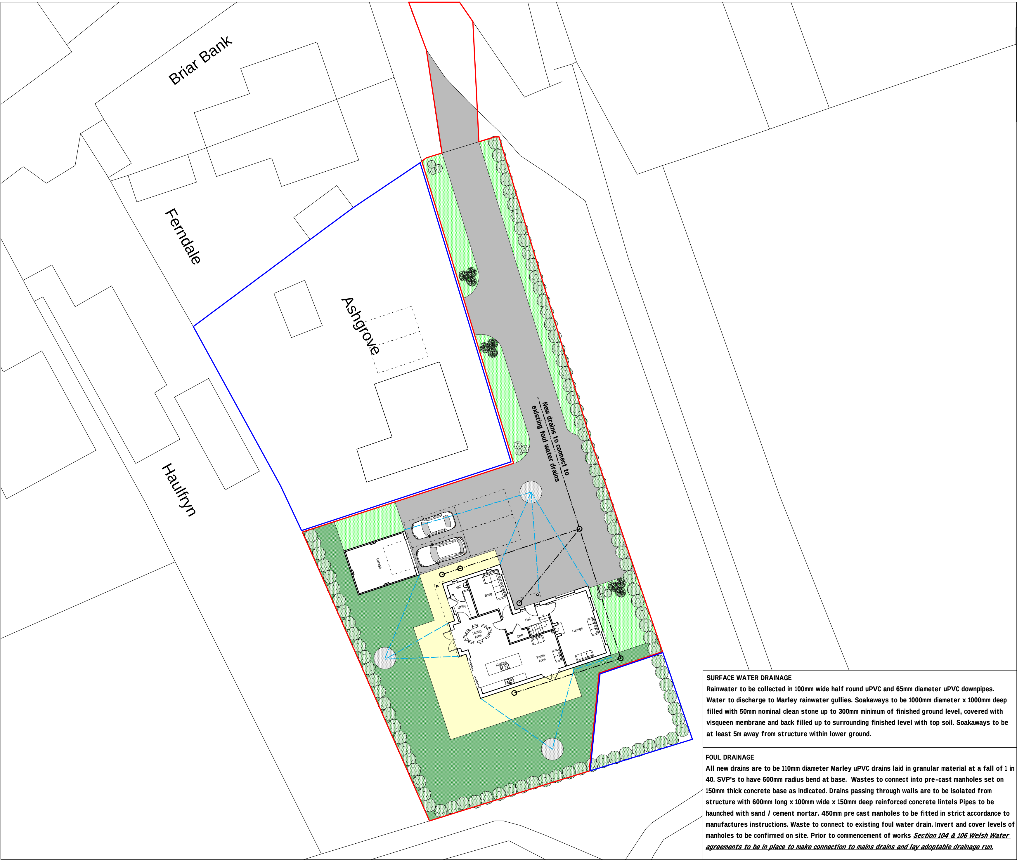
Indicative Drainage Plan 1:200
