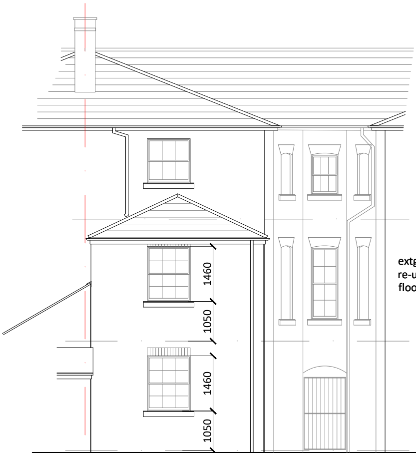
REAR ELEVATION extg window re-used to first floor rear elevation.
