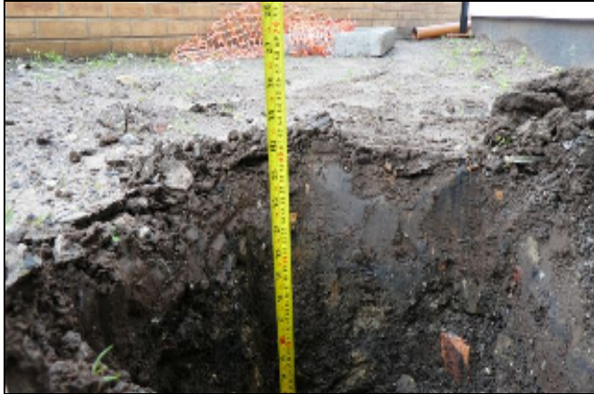
Plate 3 – Barrier layer depth 620mm
