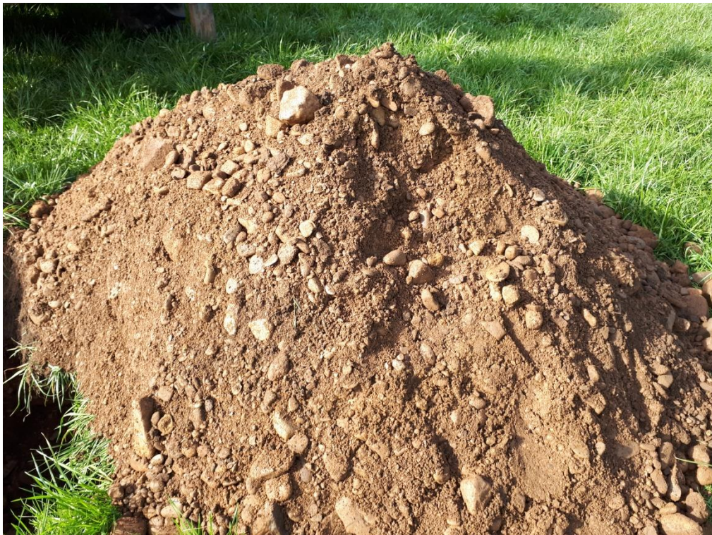
Trial Pit 06 – Arisings
