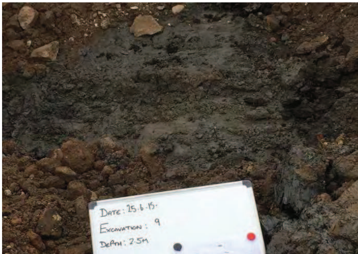
Photo (28): Base of Excavation Area 9 – visually unimpacted clay encountered at 2.5m
