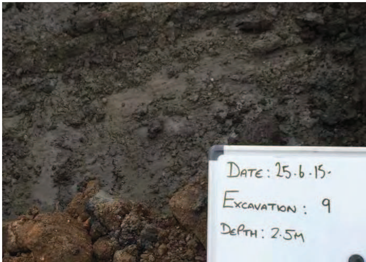
Photo (29): Base of Excavation Area 9 – visually unimpacted clay encountered at 2.5m
