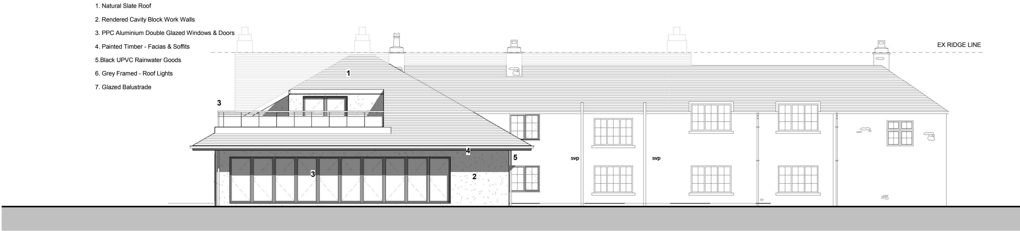
North West Elevation 1 : 100
