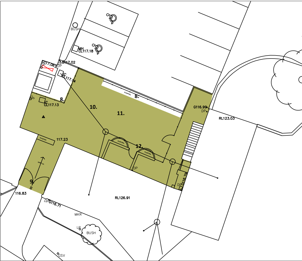
SITE PLAN - REAR ENTRANCE/DRAINAGE & PAVING SCALE 1:200
