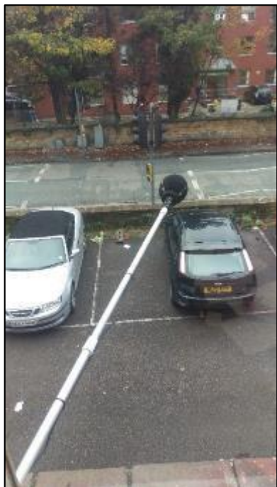
Figure B1: SLM from inside building
