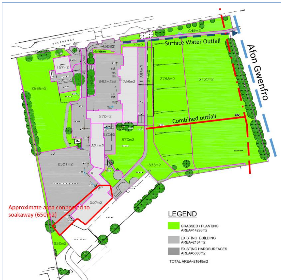
Plan showing existing permeable and impermeable areas
