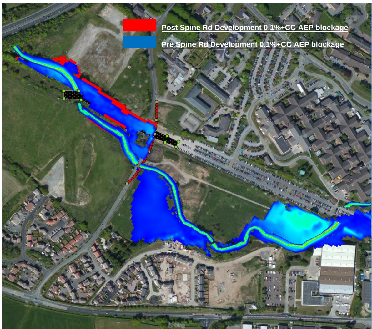
Figure 4-4 – 0.1%+CC AEP blockage 67% disused railway culvert pre and post spine road development
