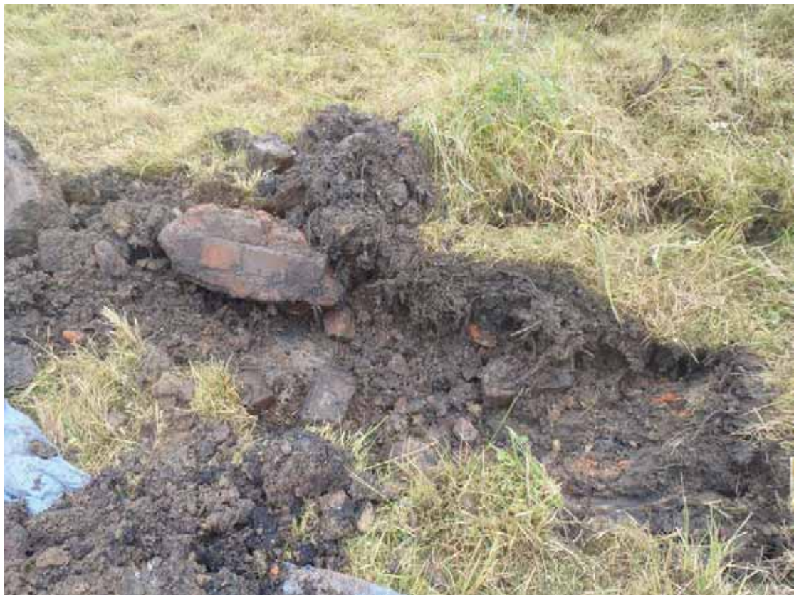
TP22: Showing blacked Made Ground immediately below thin top soil
