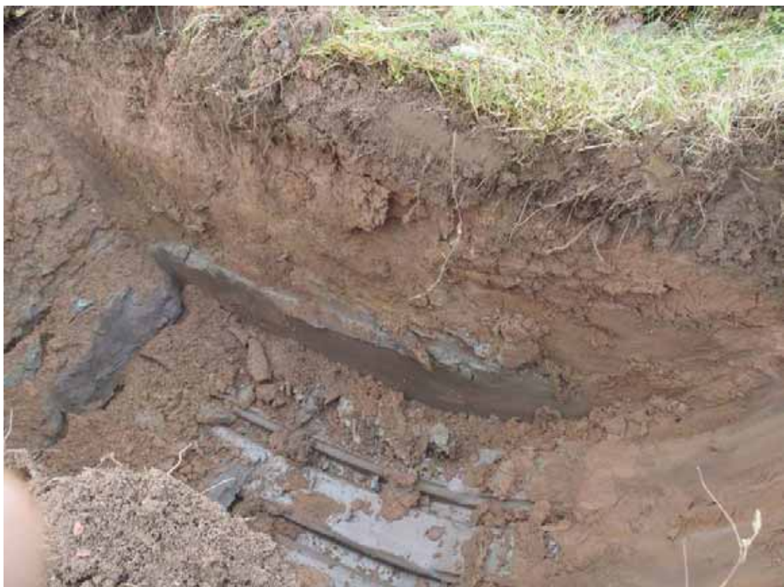
TP12: Showing sandy clay (alluvium) at base of trial pit with overlying sands (alluvium)
