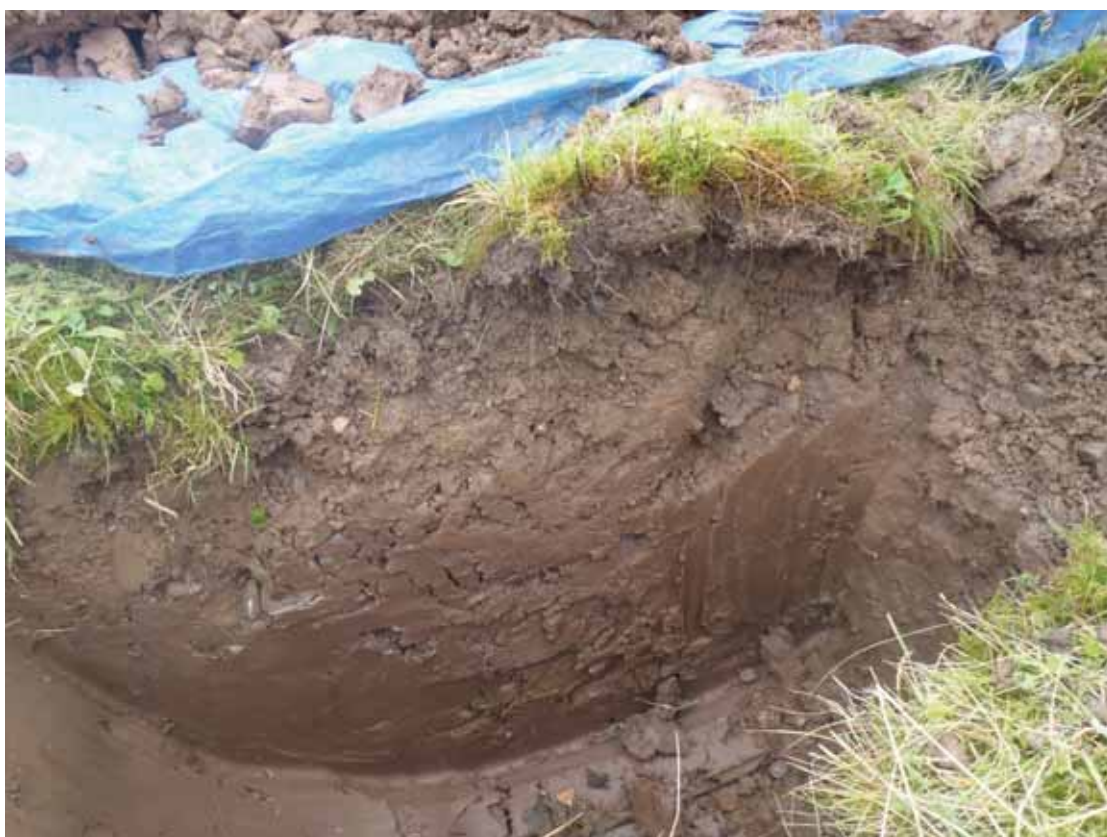
TP6: Showing 0.3 m of clayey Made Ground over glacial till
