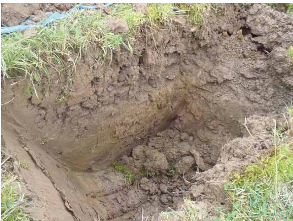
TP15: Showing clayey Made Ground to 0.6 m overlying sandy clay (alluvium)
