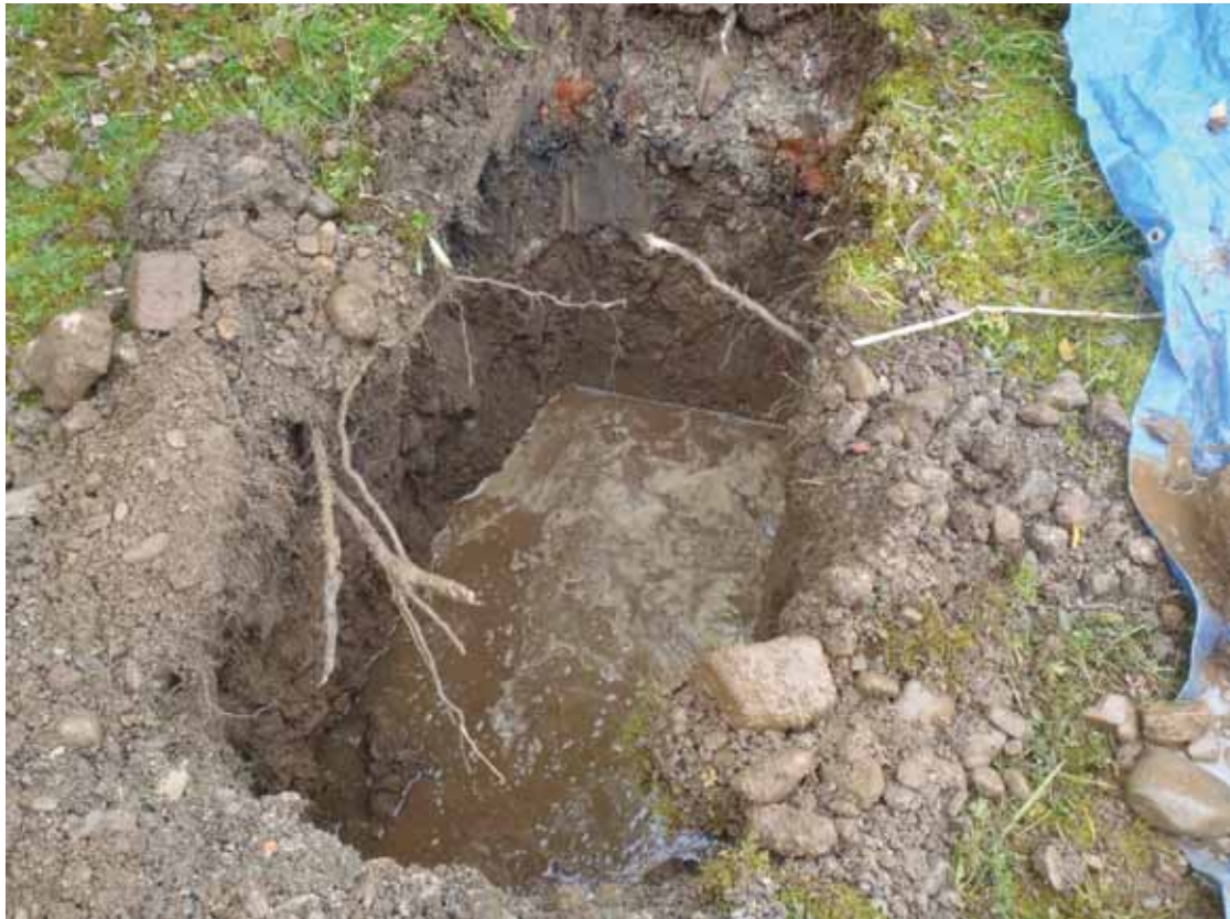
TP4: Showing water at base of trial pit
