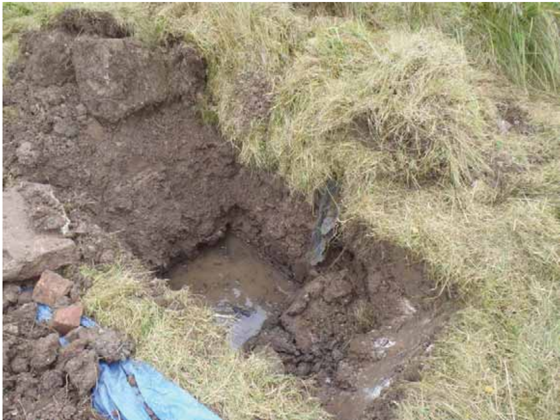
TP20: Showing water strike at 1 m
