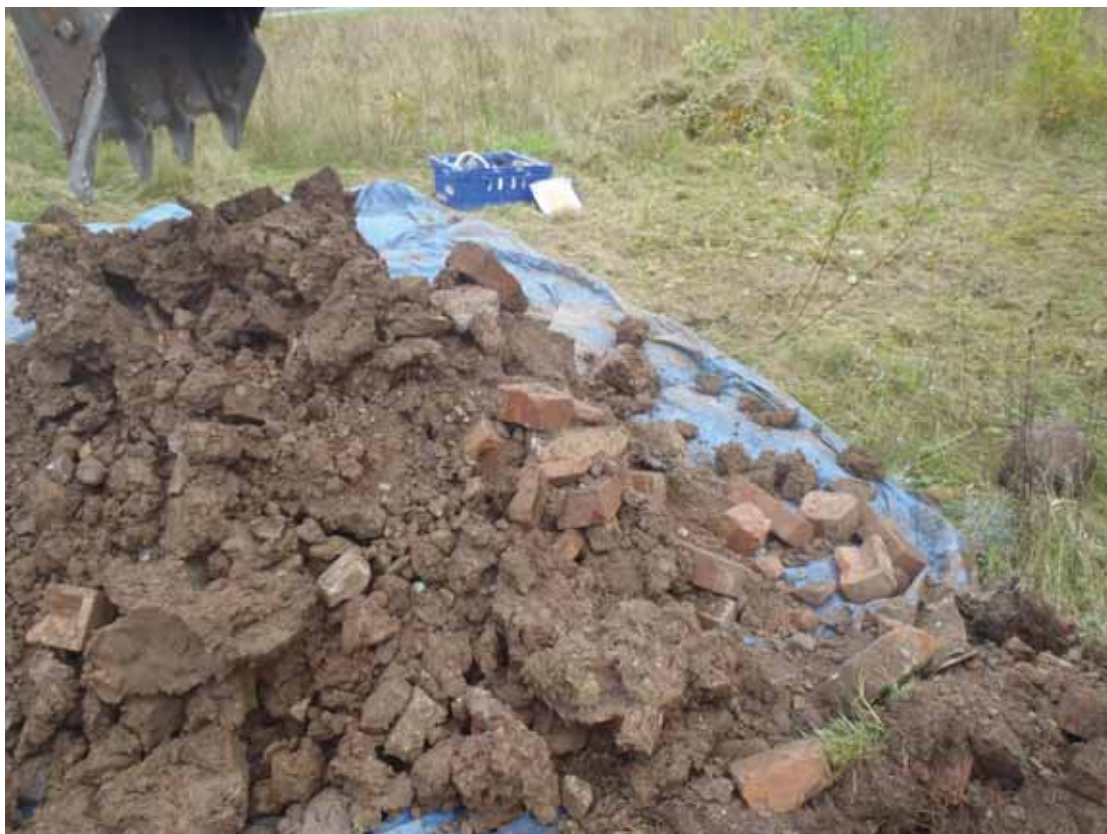
TP5: Showing clayey Made Ground with significant quantities of brick
