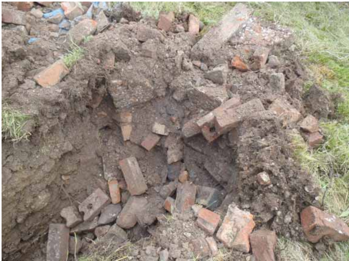
TP5: Showing southern end of trial pit with typical demolition rubble (concrete / brick)
