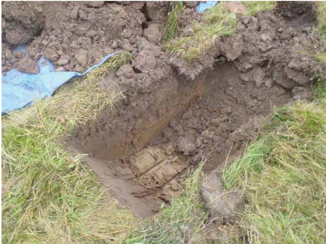
TP28: Showing 0.4 m sandy Made Ground with occasional plaster overlying silt / clay (alluvium)
