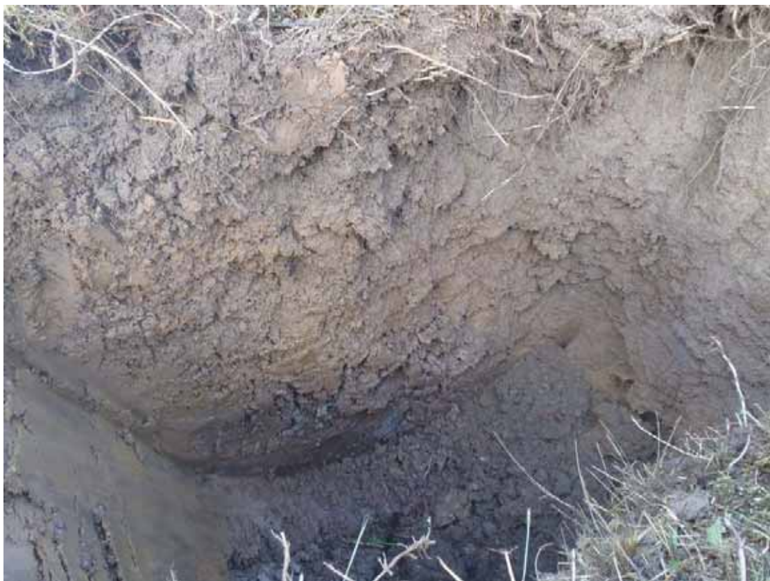
TP13: Showing clayey Made Ground to 0.7 m overlying sandy clay (alluvium)
