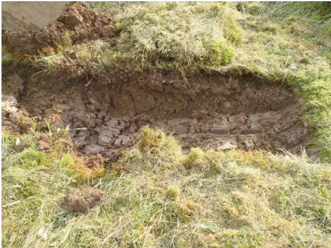
TP8: Showing glacial till immediately below thin top soil
