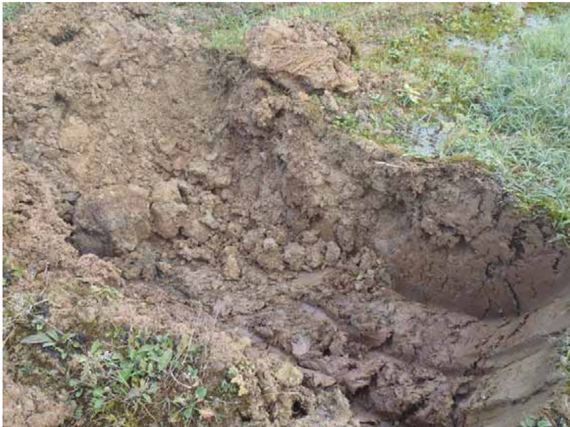
TP11: Showing glacial till immediately below thin top soil
