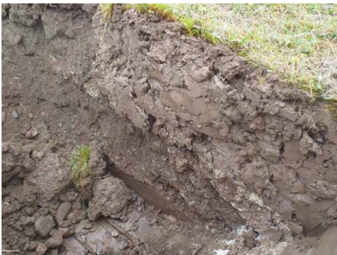
TP26: Showing clayey Made Ground with occasional plaster overlying silty clay (alluvium)
