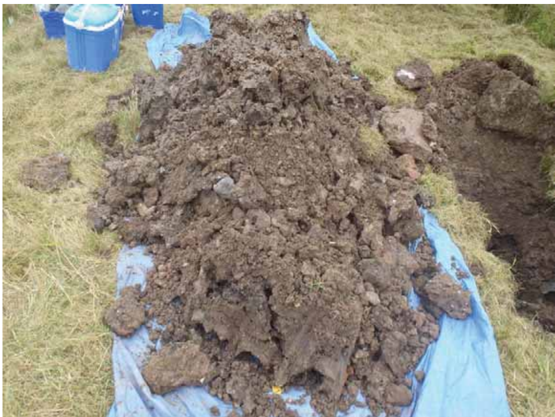
TP20: Showing Made Ground from trial pit
