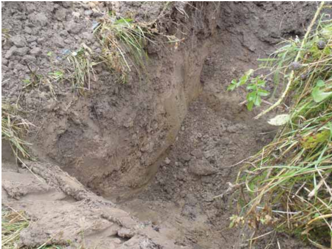
TP34: Showing 0.4 m layer of clayey sandy Made Ground above sand (alluvium)
