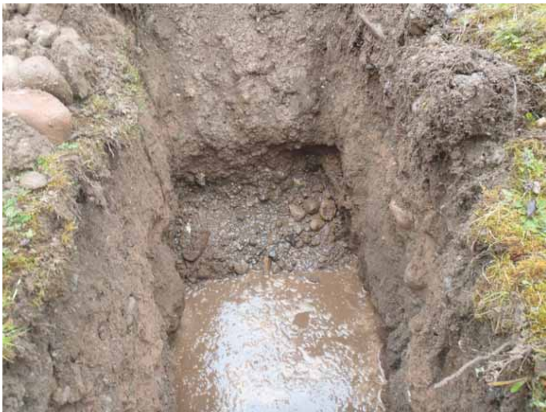
TP38: Showing dense gravel and cobble backfill with water strike at 1 m
