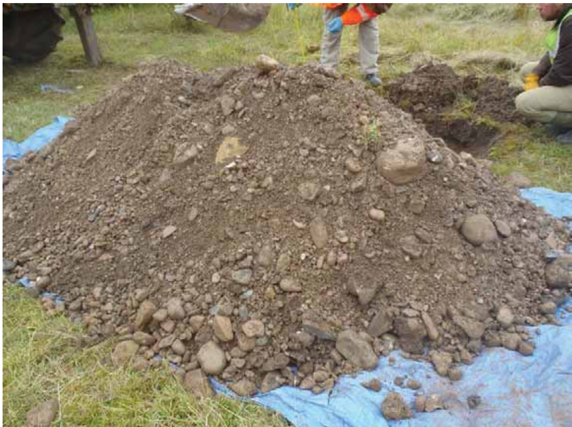
TP23: Showing general view of dense gravel and cobble backfill (similar material also observed in TP4 and TP38)
