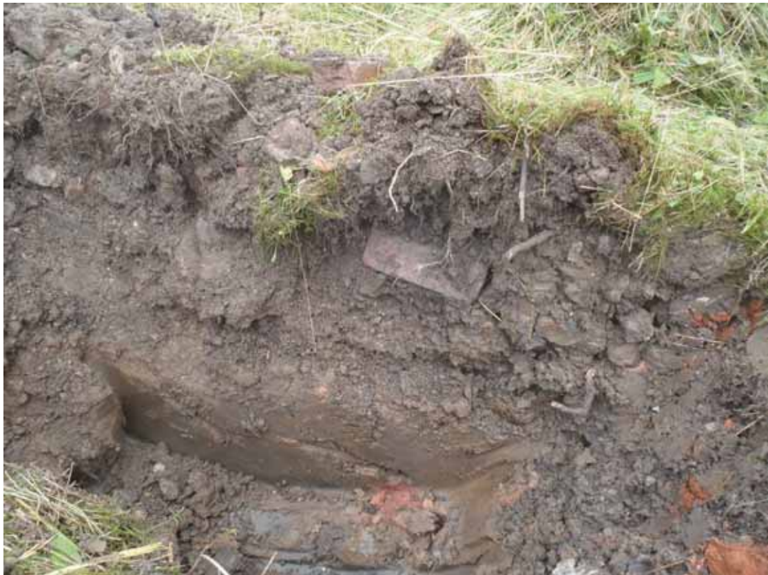
TP2: General view of trial pit showing 0.9 m of Made Ground over glacial till
