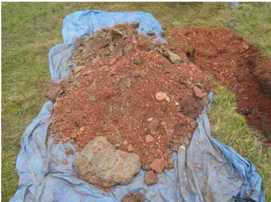
TP29: Showing 0.25 m layer of 'burnt shale' encountered above silt (alluvium)
