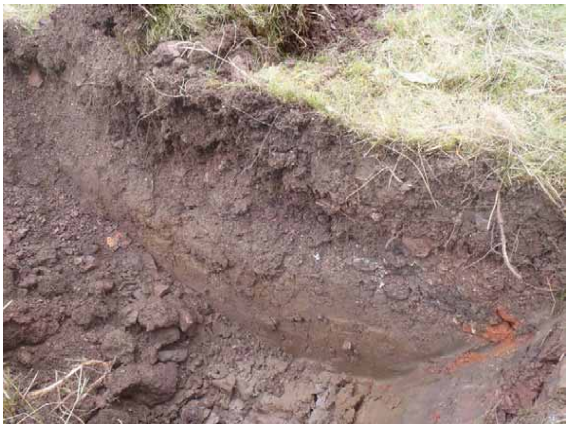
TP20: Showing Made Ground with ash, plastic and tarmac
