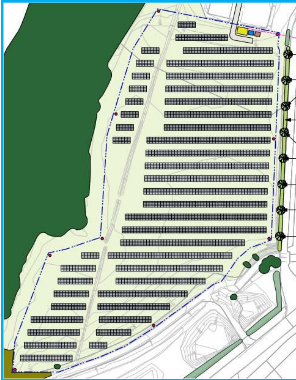
Fig 7 Plan of proposed solar farm. Arrays are indicated in black and perimeter fence in blue. Note the utility ridge is avoided (in grey) running north-south through the site. Also note creation of new hedge with trees to the east.
