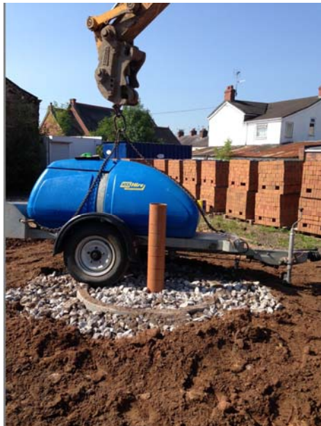
Photo 1 – Soakaway test location
