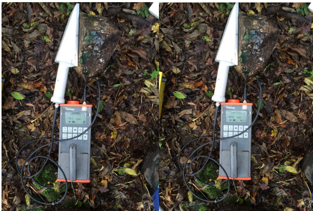
Figure A10 Elevated beta and alpha count rates from naturally occurring radioactivity in a ceramic glazed brick.
