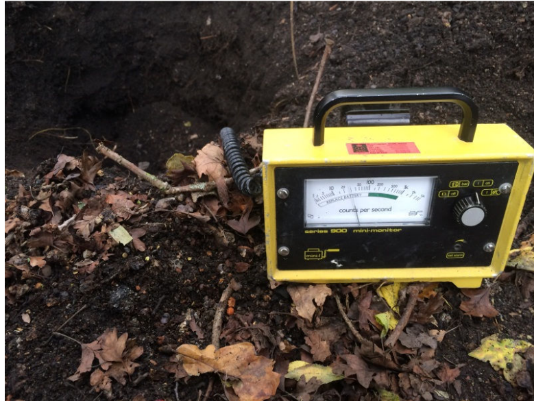
Figure A9 Slightly elevated count rates due to naturally occurring radioactivity in ash.
