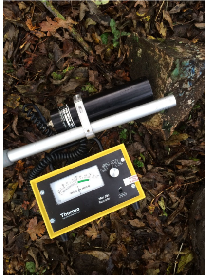
Figure A11 Elevated gamma count rates from naturally occurring radioactivity in a ceramic glazed brick.
