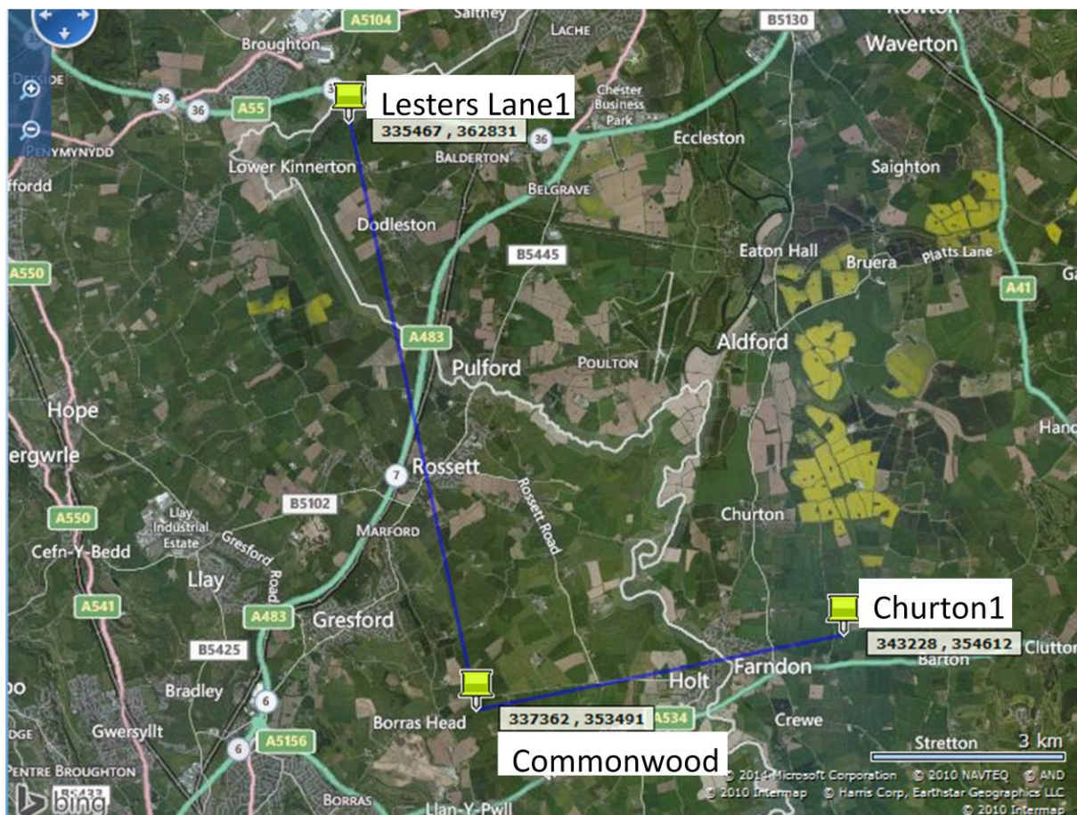
Figure 4: Map showing previously drilled exploratory CBM boreholes in the area by DART Energy (Churton1) and Green Park Energy (Lesters Lane1). Does not include further planned sites, well locations from DECC.
