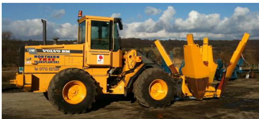
A loader and tree-spade similar to that to be used for the translocation.
