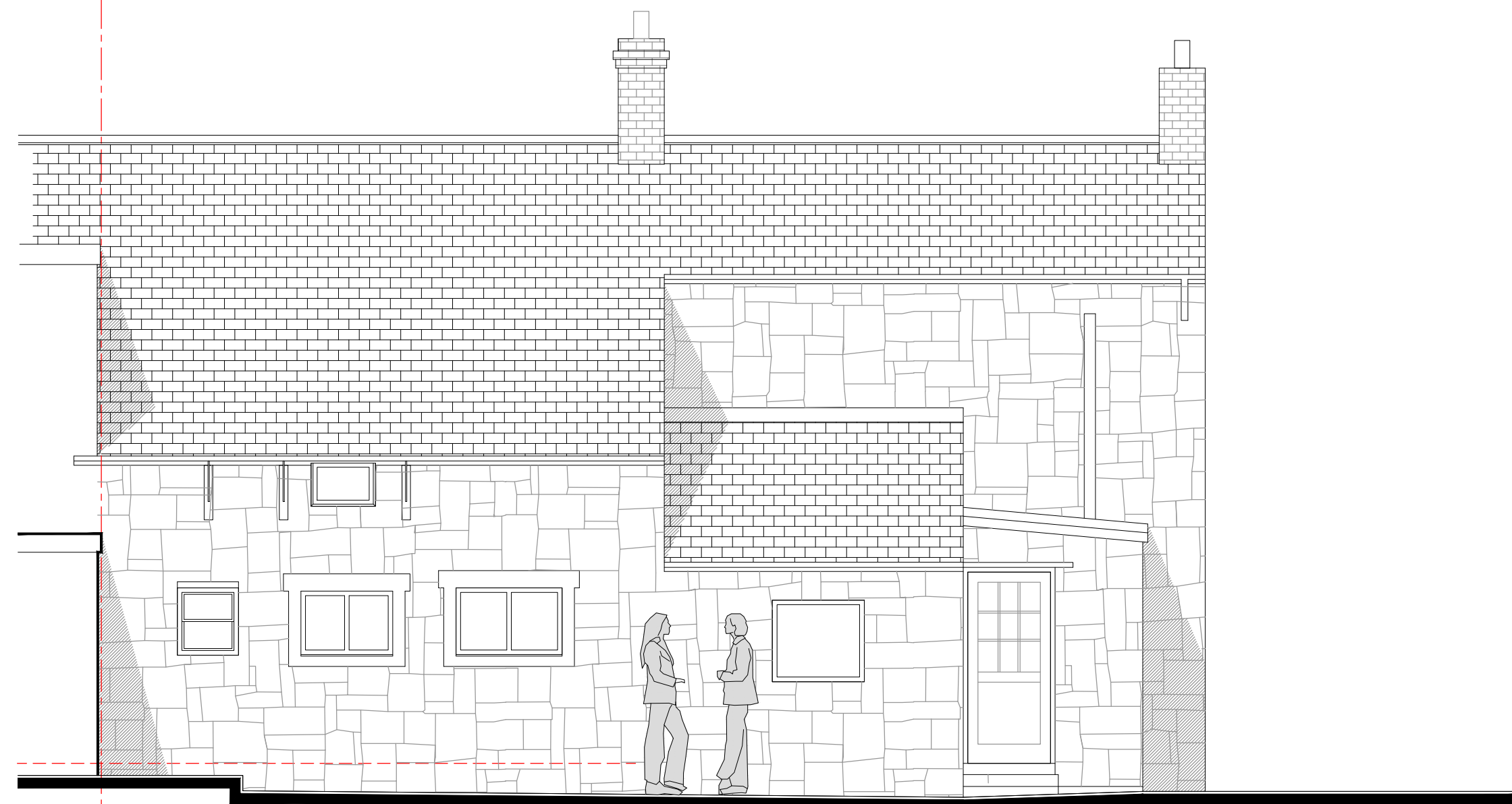
Existing Rear Elevation 1:50
