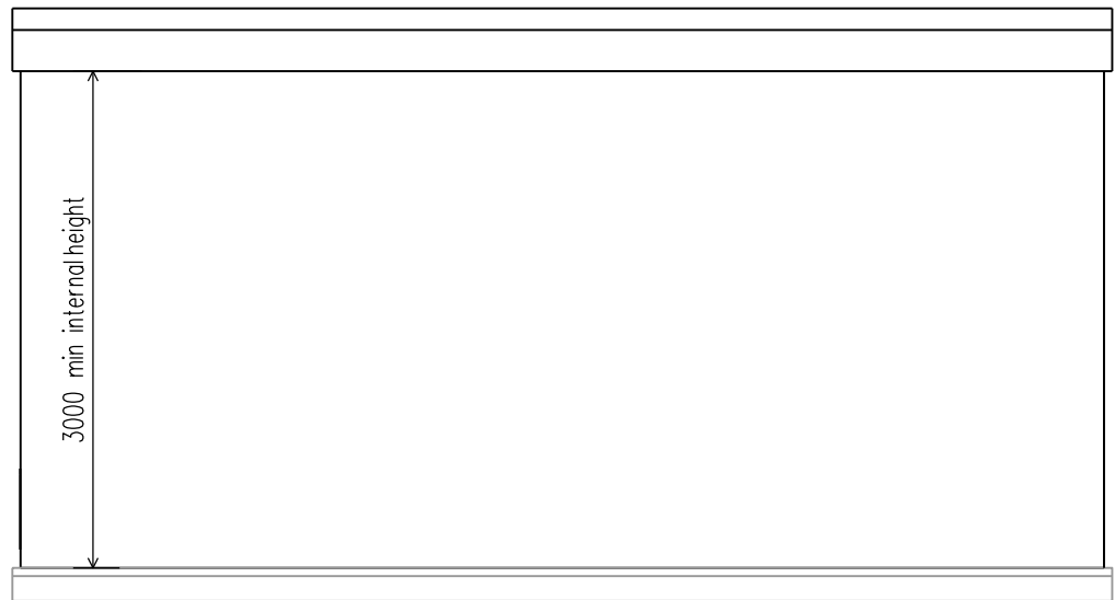
AHU Enclosure Elevation C
