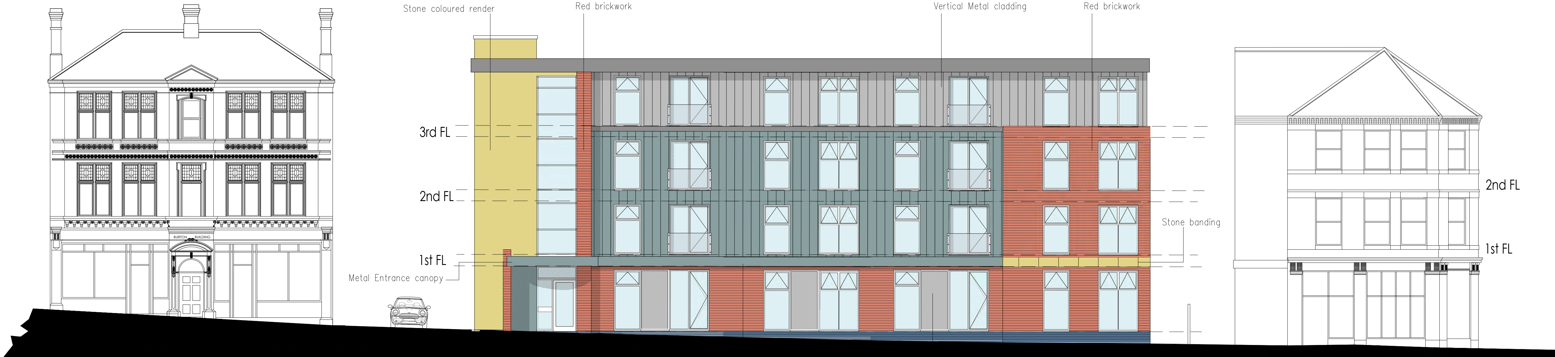
PROPOSED FRONT ELEVATION TO BRIDGE STREET. 1:100
